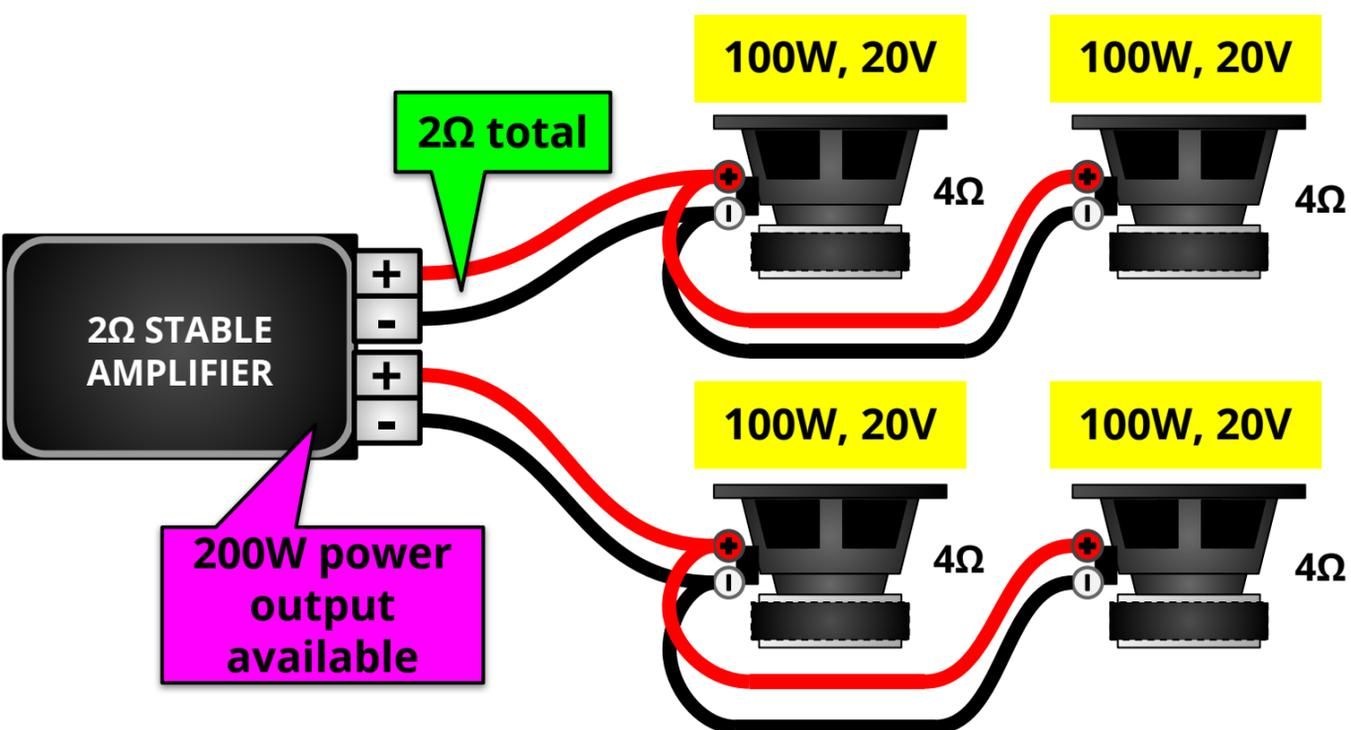
With speakers in parallel (at the min. supported Ohms load) the amp can supply its maximum power. Each speaker receives 1/2 of this power. The same output voltage is shared by each speaker when connected in parallel.
