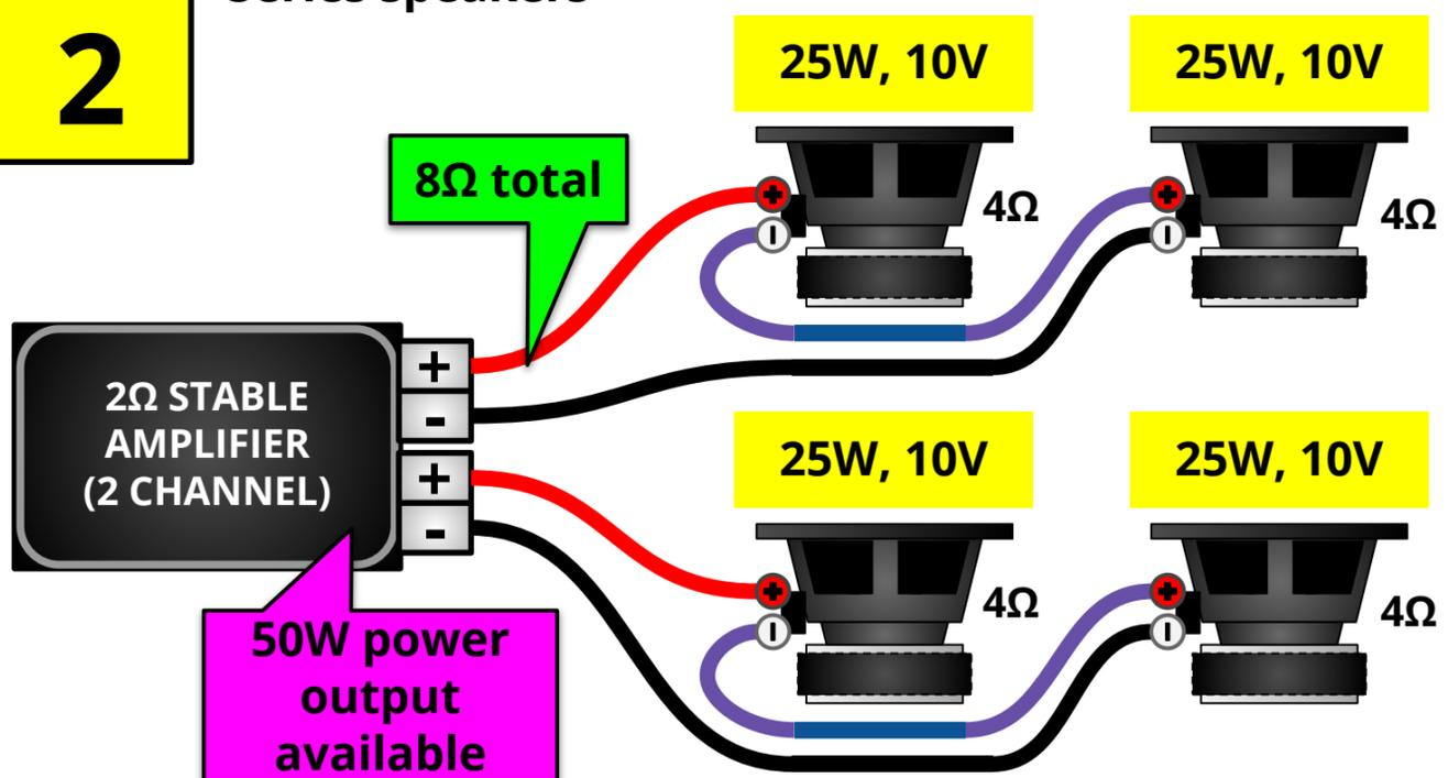
Speakers in series add together. In this example, two 4Ω speakers add up to an 8Ω load for the amp. If we know the amp can put out up to 20V, the power the amp is putting out is then:
