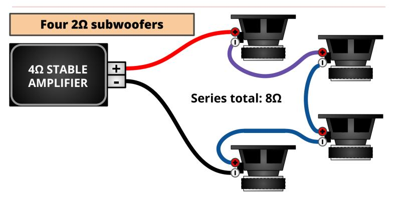
**Result:** NOT RECOMMENDED - The amp's power output will be  $\frac{1}{2}$  that of it's  $4\Omega$  rated power. Each speaker will receive  $\frac{1}{4}$ th of that, meaning minimum power developed across each. This is the only way to wire  $4x 2\Omega$  SVC speakers if needed but isn't ideal for power.
