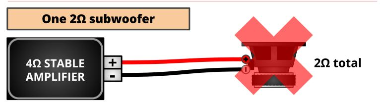
A 2 $\Omega$  SVC speaker cannot be used with an amp channel rated for 4 $\Omega$ . This will cause the amp to overheat and shut down or possibly burn out the channel outputs.
