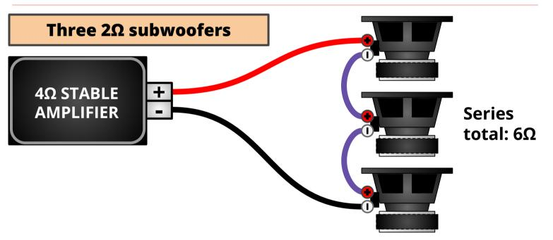
**Result:** NOT RECOMMENDED - This will reduce the total power delivered from the amp. Each sub will then have  $\frac{1}{3}$  of that power. However, you cannot wire  $3x 2\Omega$  SVC subwoofers otherwise. This works if you need to use 3 speakers but is not ideal for power.
