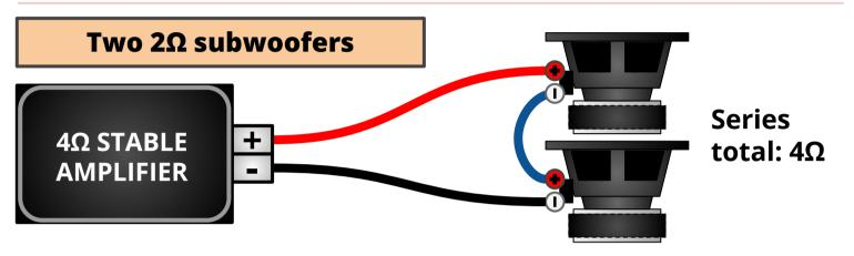
**Result:** OK - This will deliver the maximum rated power from the amp. Each subwoofer gets ½ of the max. rated power output.
