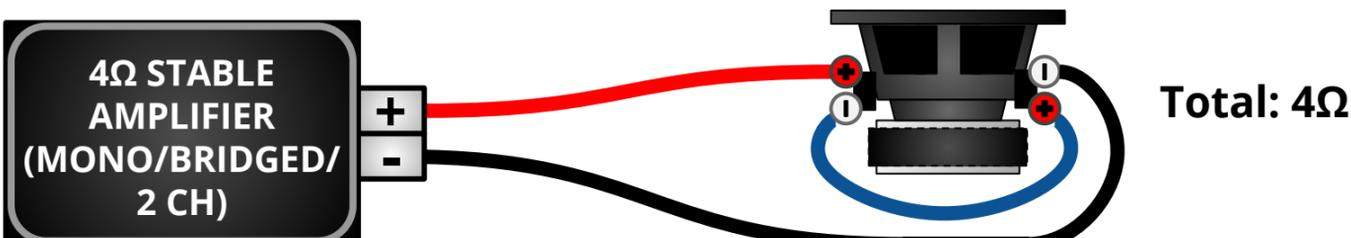
**Result: GOOD** - The subwoofer will have the full power output available from the amp. Both coils will share the power and run cooler than using one voice coil alone.
