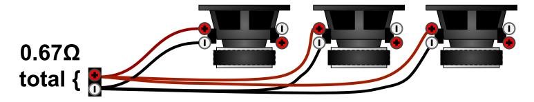
Triple subs, series-parallel voice coil example
