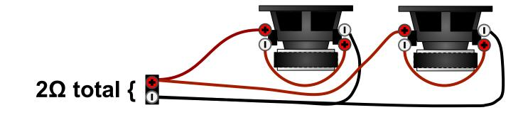
Triple subs, (single) parallel voice coil example
