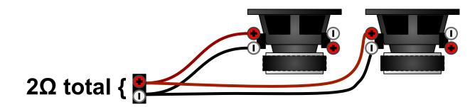
Dual subs, parallel-parallel voice coil example
