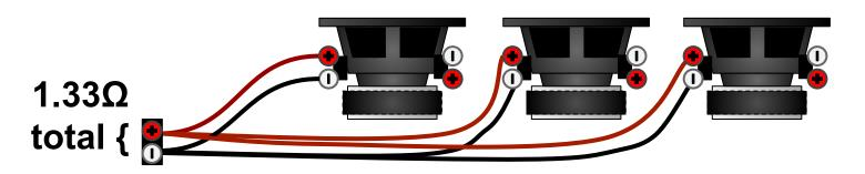
Triple subs, series-parallel voice coil example
