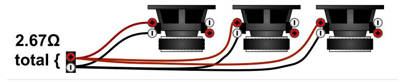
Triple subs, series-parallel voice coil example
