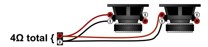
Dual subs, parallel-parallel voice coil example
